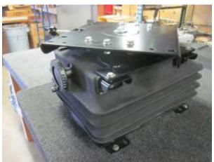
Rotate Swivel to give access to the bolt holes when installing both the swivel to the HDMS and the seat with slider to the swivel
